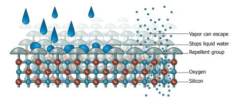
Silicone paint cures with water in the atmosphere (humidity) to form a 3-dimensional quartz-like structure of alternating silicone and oxygen atoms. Water repellent groups line the pores of the paint and stop the ingress of liquid water but allow water vapor to outgas. This structure, unique to silicone paints, invented in Germany in 1963, is the key to their performance.
