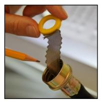
Installing silver-plated cloth (attached to hose washer) in the cold water supply hose.
